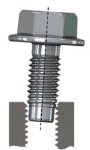
Misaligned axis (helix) of the MAThread<sup>®</sup> to the female thread.
